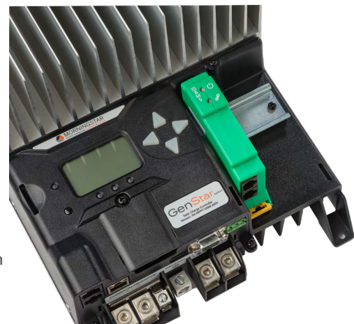
ReadyBMS installed in a GenStar MPPT charger
